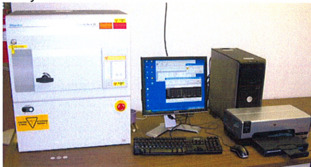
Calgary Rock's new "state-of-the-art" Rigaku Miniflex II X-ray diffractometer. Jade software with a database of over 100,000 compounds is used to evaluate mineralogy of unknown samples.
