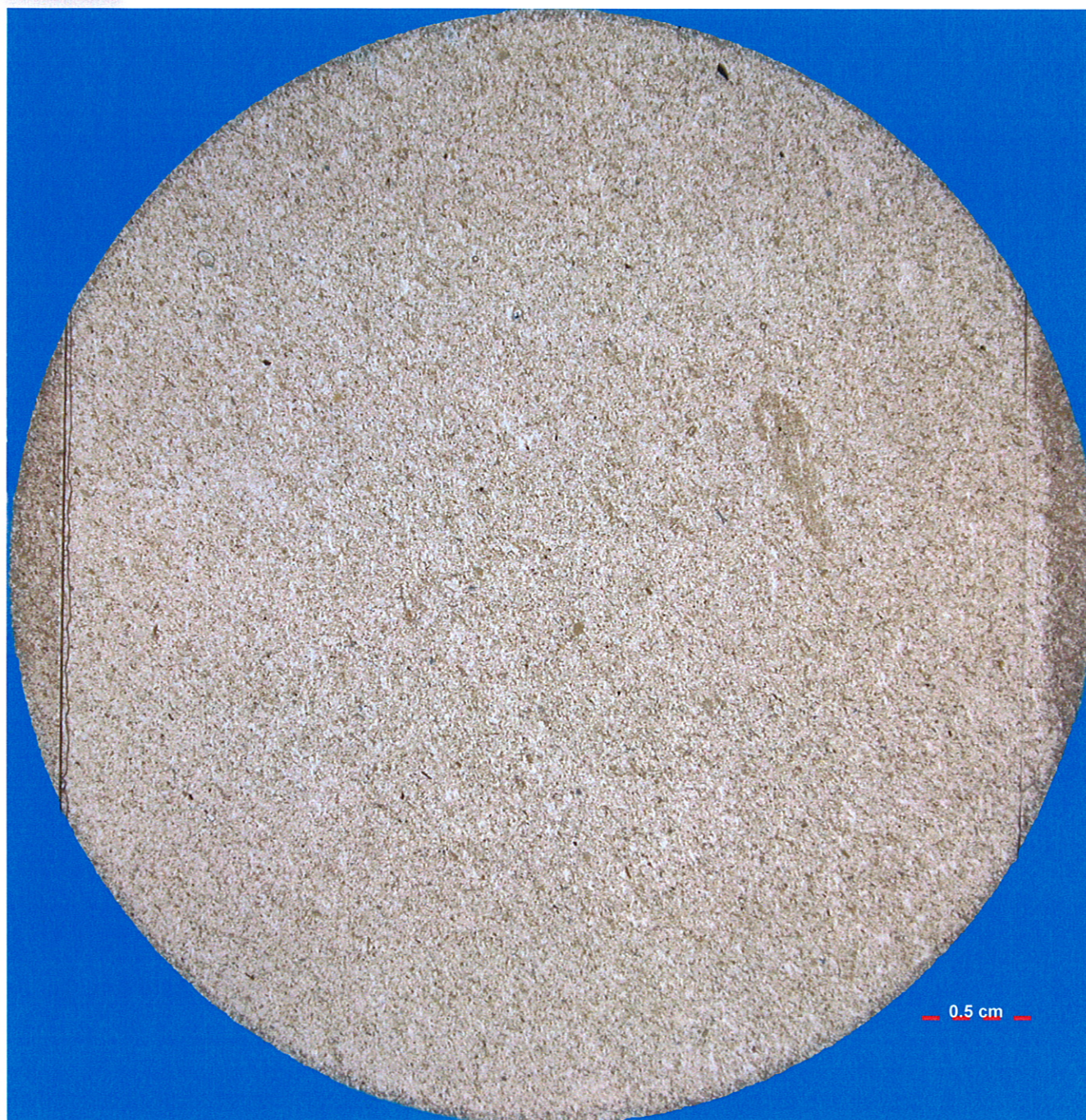
A. Moderately well sorted, silt to mid-very fine grained argillaceous litharenite.
