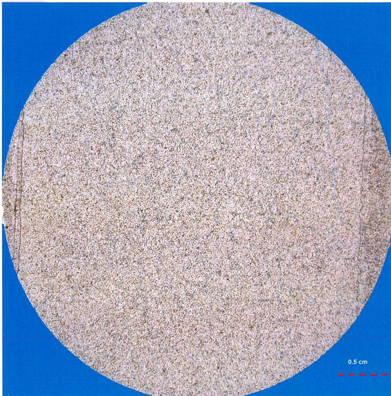
A. Moderately well sorted, silt to mid-very fine grained argillaceous litharenite
