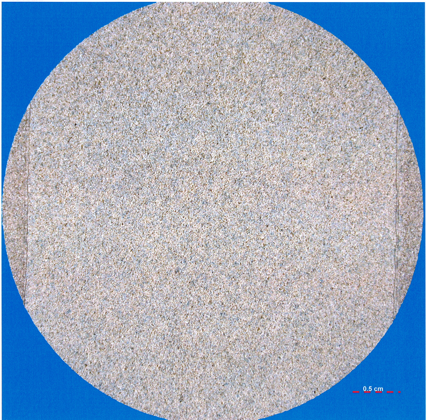
A. Moderately well sorted, silt to lower very fine grained argillaceous litharenite.
