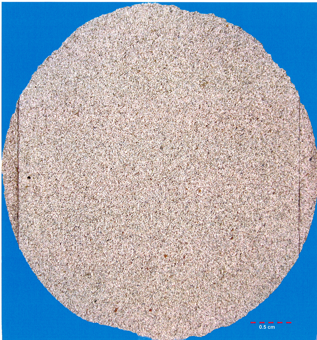
A. Moderately well sorted, silt to lower fine grained argillaceous litharenite.
