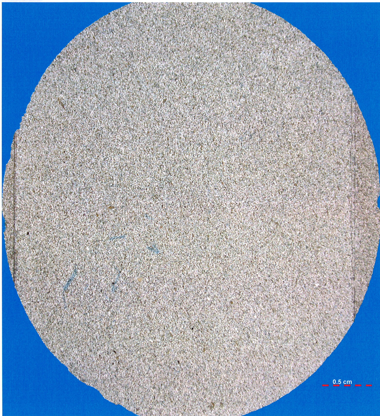
A. Moderately well sorted, silt to lower fine grained argillaceous litharenite.
