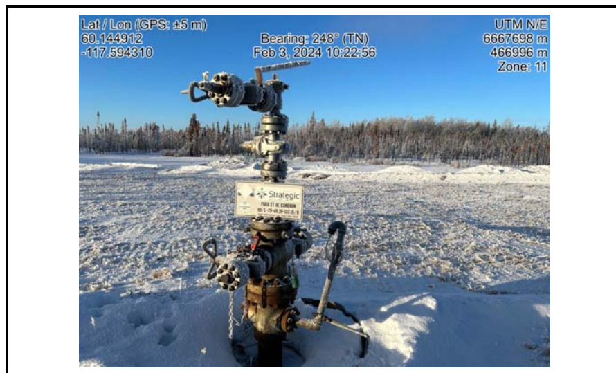
L-29 Wellhead, Bubble test in progress
