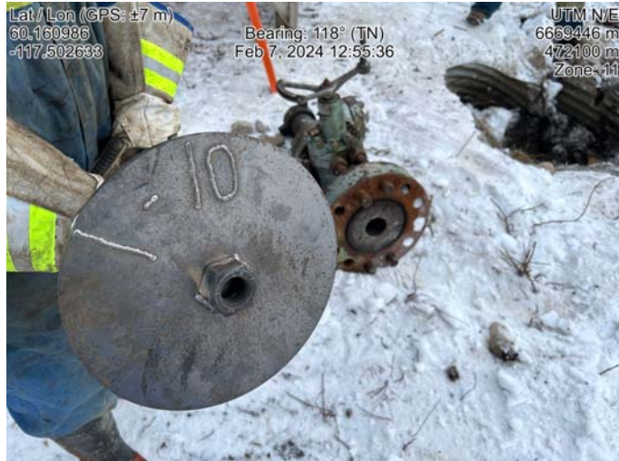
The vented cap with "I-10" Welded in place
