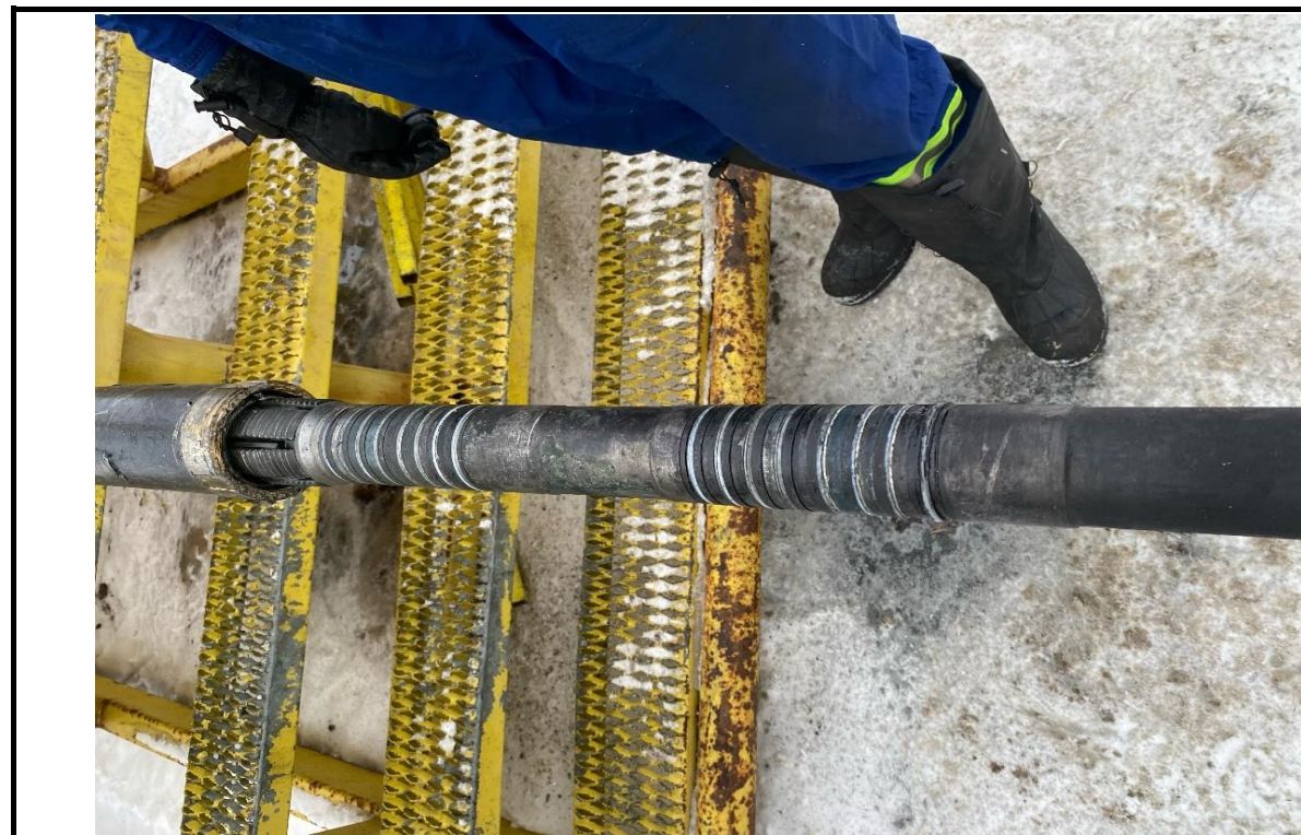
March 7 - Recovered the packer mandril and sealing elements
