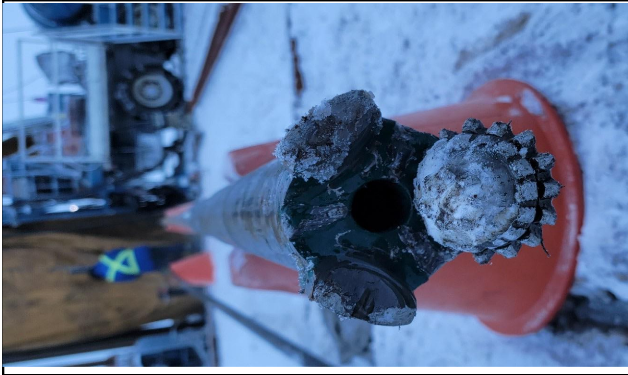
Jan 30th - Tricone bit missing 2 of its cones
