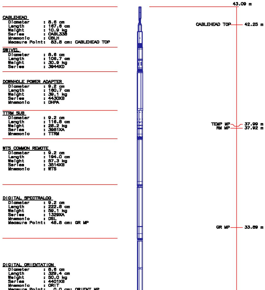
ARRAY ACOUSTI LOG ELECTRONICS, B CHANNEL
