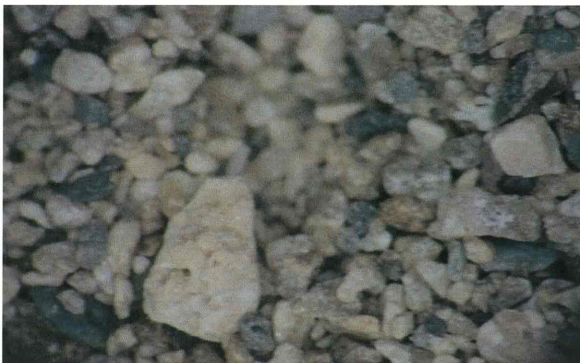
Sul Pt. Dol. 1520-1525mMD-Build Sec. 2H-03-Vuggy Porosity
