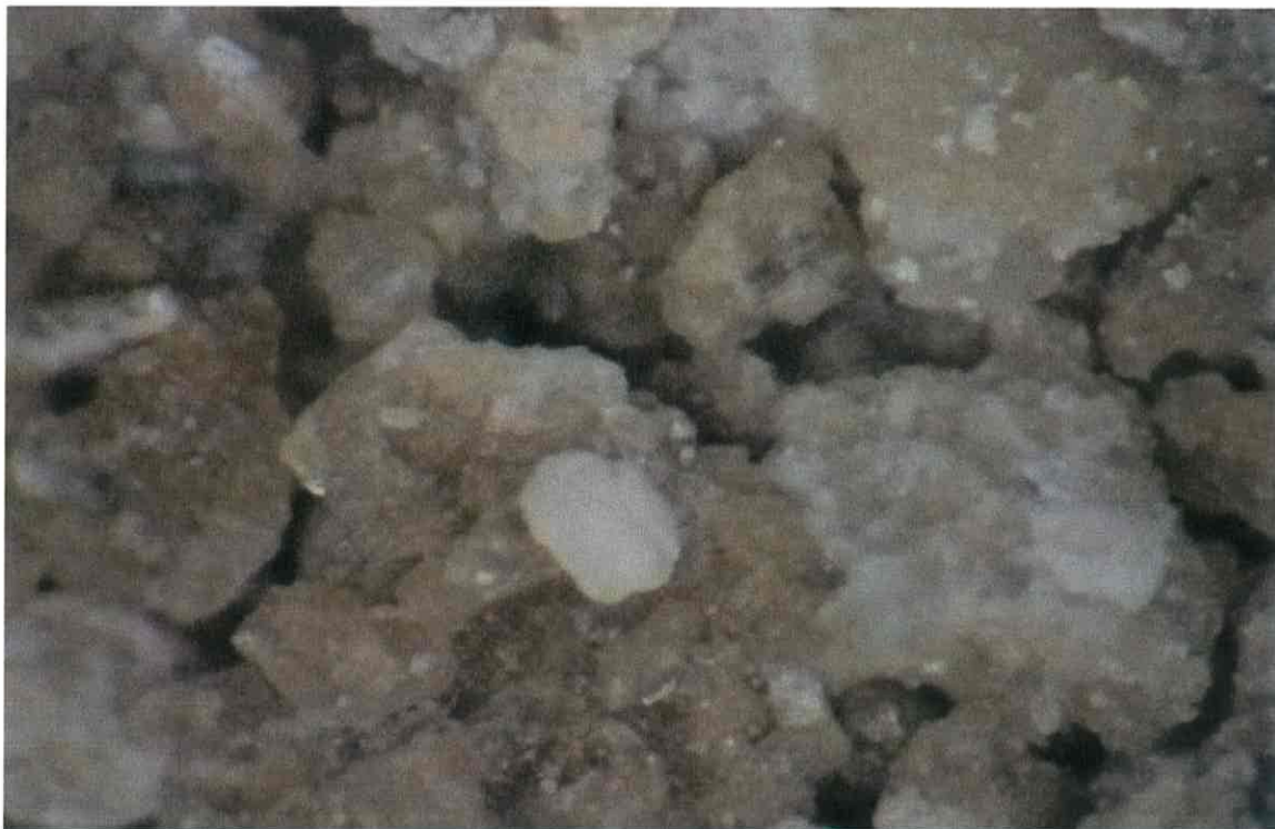
Sul Pt Dol 2485-2490mMD Hor Sec 2H-03-Free crystals and Vugs
