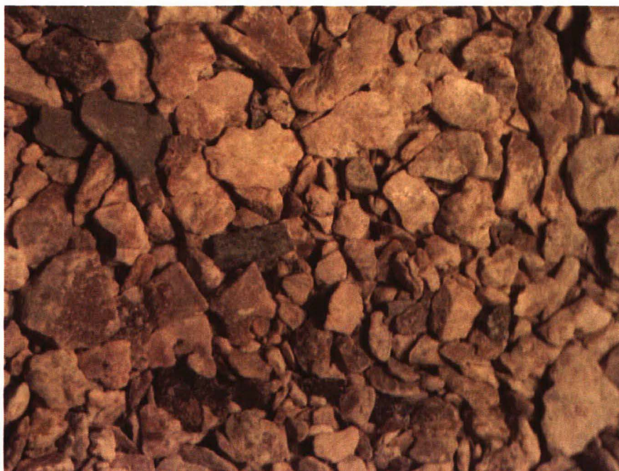
UPPER SLAVE POINT massive chalky flaky limestone, 1315m, 20X zoom
