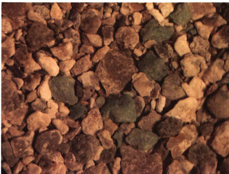
WATT MOUNTAIN green waxy calcareous pyritic shale, 1350m, 20X zoom
