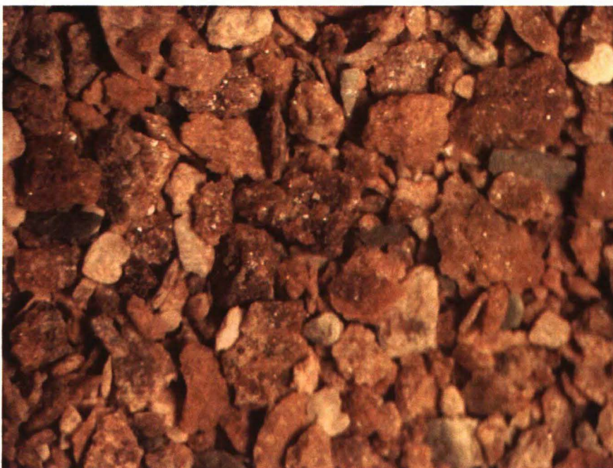
SULPHUR POINT DOLOMITE, fine crystalline grainstone, 9-12% porosity, 1375m, 20X zoom
