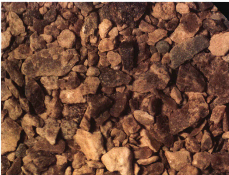
LOWER SLAVE POINT in part resinous, bituminous, anhydritic limestone, 1335m, 20X zoom
