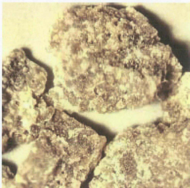
1375m porous Slave Point limestone
