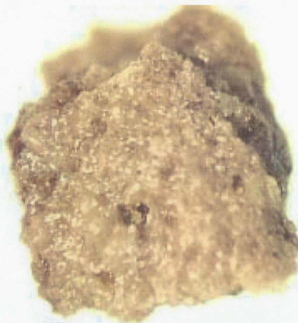
1419m porous Sulphur Point dolomite
