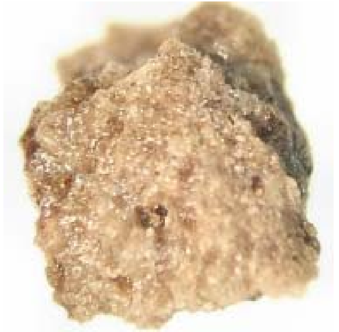
1419m porous Sulphur Point dolomite
