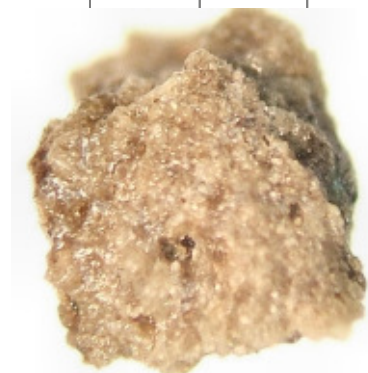
Picture of Sulphur Point Dolomite Magnification power 20X 1418m - 1420m
