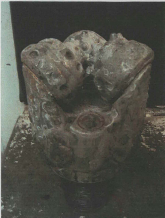
Bit #2, Smith Tool, F12Y Drilled 1108 to 1455 = 347m in 41.25 hrs
