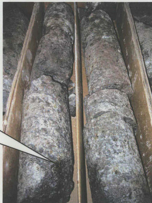
Vugs & Dol rhombs lining fracture surface
