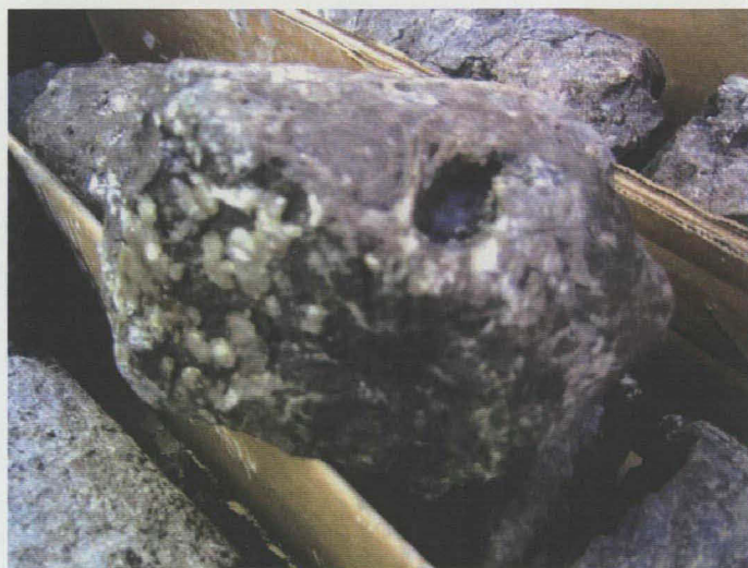
Vugs & Dol rhombs lining fracture surface
