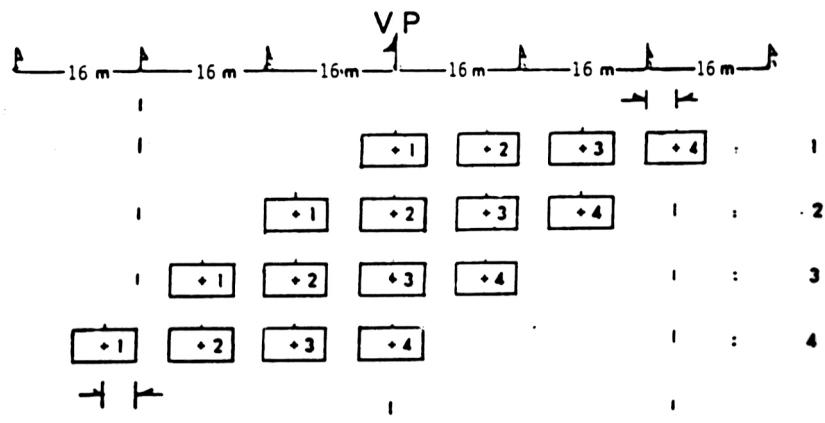
VIBRATORS stacked Bumper-to-Bumper, IN-LINE, Maximum distance = 2 meters.
