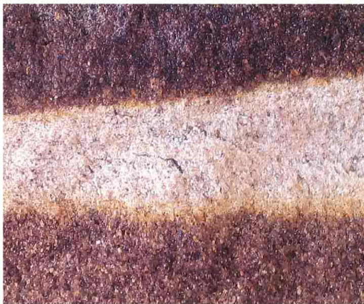
Figure 12: Detail of deformation band in Kamik C sandstone showing decreased porosity within the deformation band (white zone).
