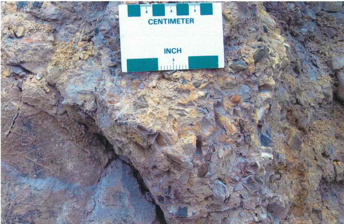
Figure 21: Karst fill at South Campbell Lake quarry. Fill consists of limestone and siltstone breccia, and is reported to contain Cretaceous fossils.
