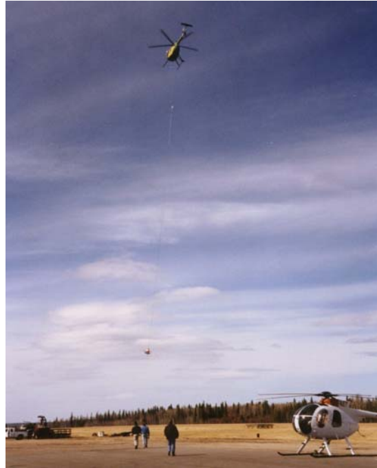
Figure 3. Hughes 500 helicopter and longline gravity meter on the 150-foot longline
