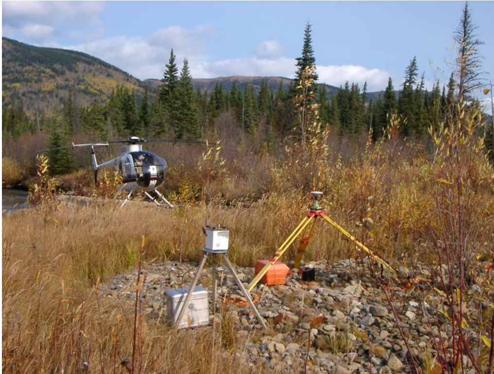
Figure 5. Typical temporary GPS control base
