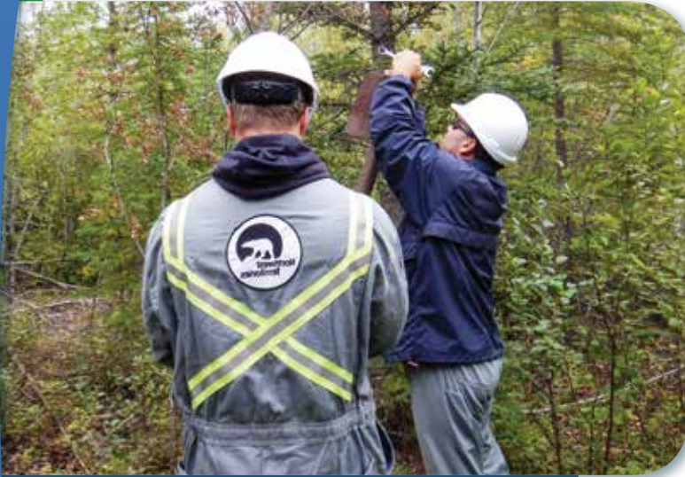
Mischa Malakoe (Technical Specialist) and Brent McGarry (Alberta Energy Regulator) installing gas sampling equipment on the marker of an abandoned well near Jean Marie River, Northwest Territories, August 2015 (OROGO)
