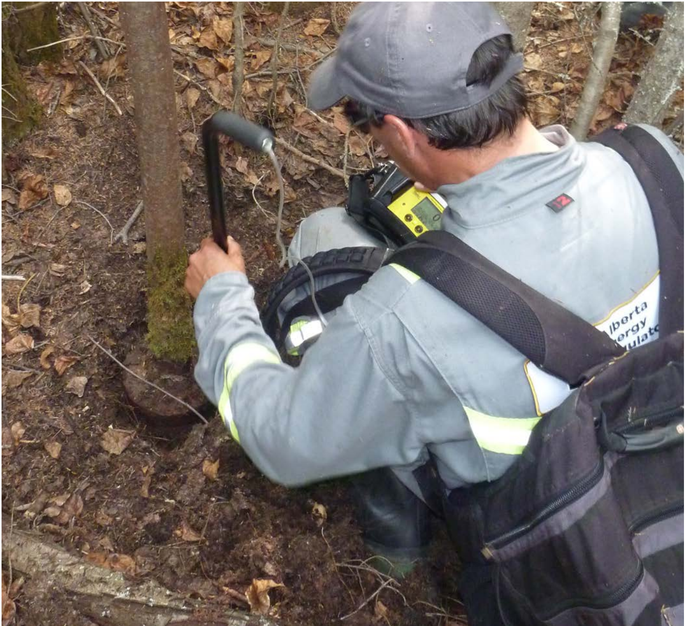
Al Duben, Air Monitoring Specialist with the Alberta Energy Regulator, using a portable methane detector to detect any leaking gas from the abandoned well. (OROGO)
